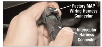
Plug the Interceptor harness connector into the factory MAP wiring harness connector, and push in the locking clip. Reinstall the engine beauty cover then the intake hose removed in the previous steps. *DO NOT reconnect the air intake sensor as it will be reconnected in the next section of the Interceptor installation.*
